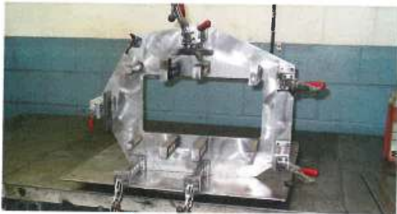
A jig or fixture must be used to restrain parts in position to control distortion during welding.
