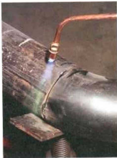
Figure 39-4. A common preheat method is to move an oxyacetylene flame over the surface of the metal.
