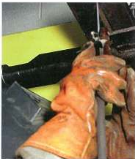
Figure 2-9. Always wear gloves when welding and cutting to protect the hands from ultraviolet rays and spatter.
