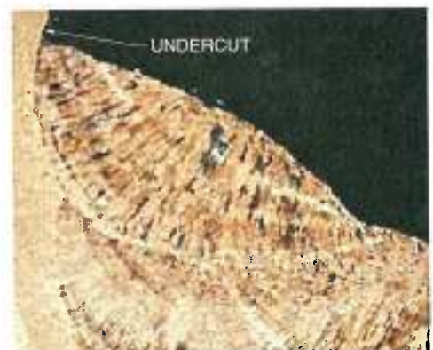
Figure 34-26. Undercut occurs when a groove is melted into the base metal adjacent to the weld toe and is left unfilled by weld metal.
