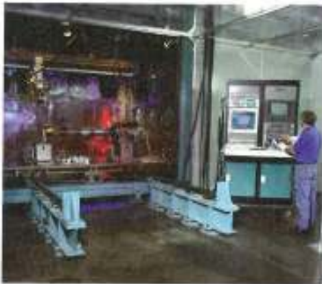
Figure 28-16. The welding gun and workpieces are enclosed in the vacuum chamber of an electron beam welding machine.
