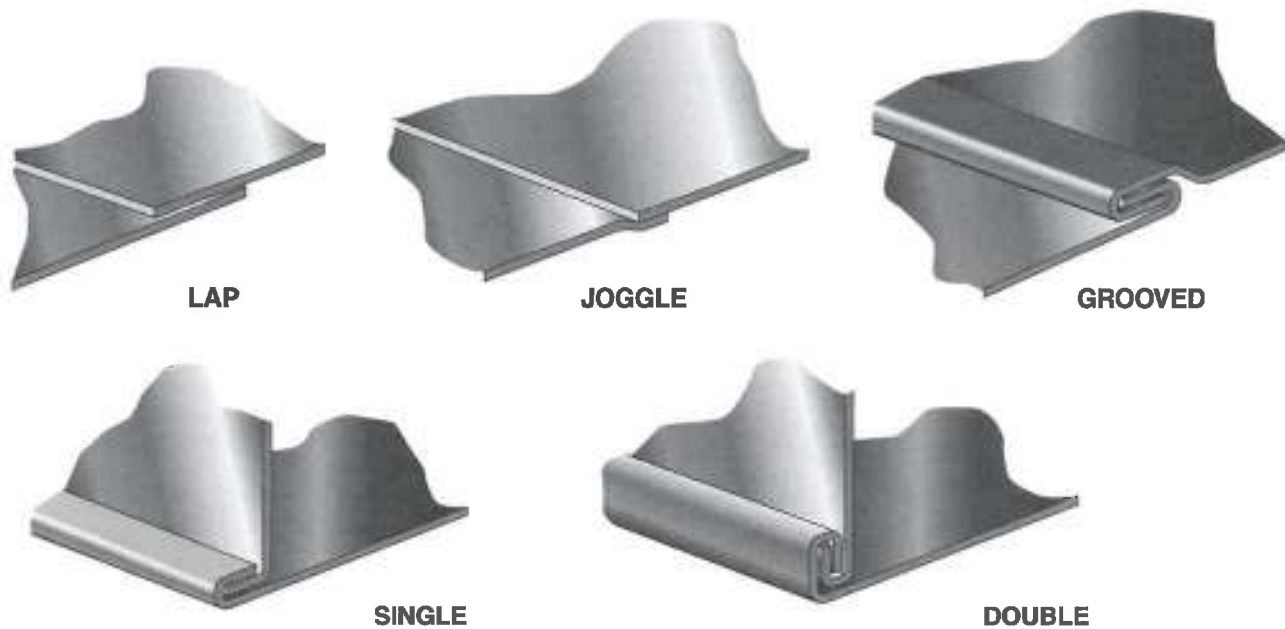
Figure 23-15. Joint designs for soldered seams are determined by the strength requirements of the joint.
