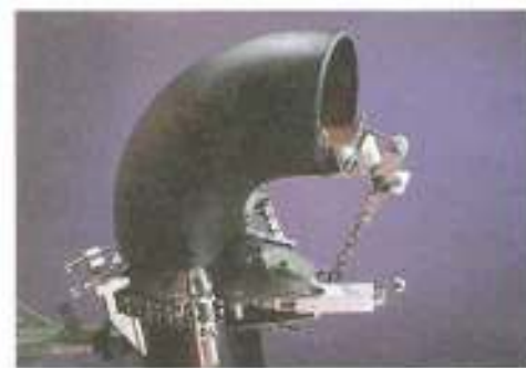
Figure 27-6. Line-up clamps hold pipe sections securely in position while tack welds are made.
