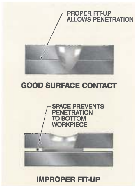
Figure 28-12. Good surface contact is important to making a sound spot weld.
