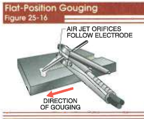
Figure 25-16. When gouging in flat position, the electrode holder is held so that the electrode slopes back from the direction of travel.
