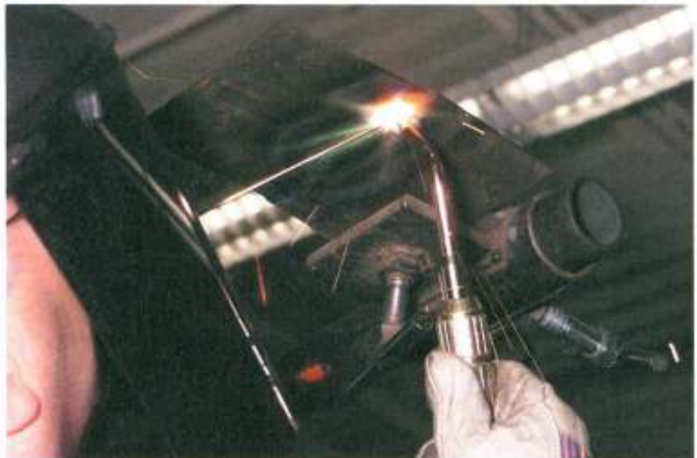
Figure 4-8. An oxyacetylene welding torch provides complete control of the flame during welding.
