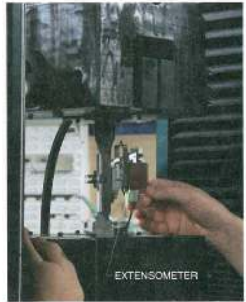
Figure 31-4. An extensometer measures the extension or elongation of the tension test specimen.
