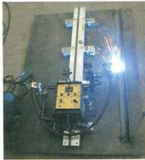
Figure 25-13. A semiautomatic plasma arc cutting unit is commonly used to ensure an even cut to the metal.
