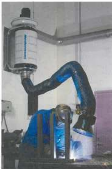
Figure 22-3. Fume extractors are commonly installed within a permanent ventilation system in a shop.
