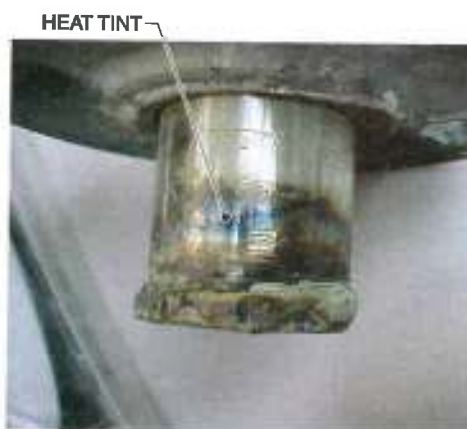
Figure 41-7. Heat tint is formed on stainless steel during welding but does not usually compromise the corrosion resistance of the stainless steel.
