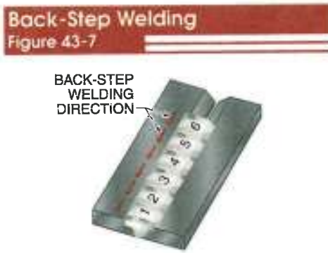
Figure 43-7. Back-step welding is a welding process in which weld passes are made in the direction opposite to the progression of welding.
