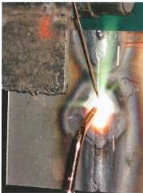
Figure 7-1. Uphill welding is performed with an uphill progression. Do not allow the weld pool to get too large.
