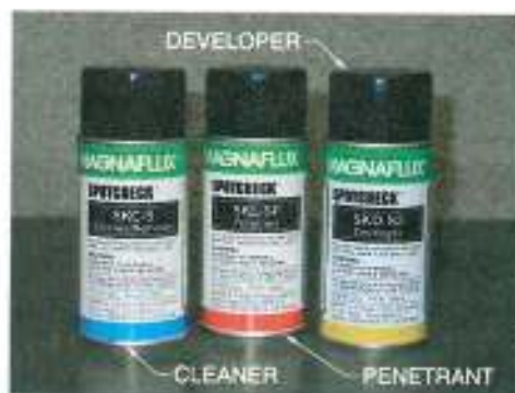
Figure 32-5. A portable visible-penetrant, solvent-removable PT kit is useful in determining indications when the testing needs to be done at a remote location.
