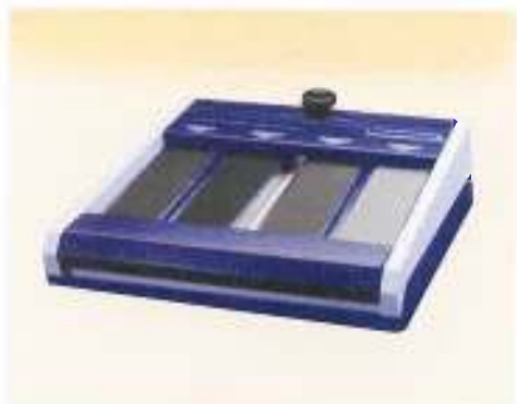
Figure 33-5. Grinding in four-stage belt grinding starts with 240-grit and finishes with 600-grit paper.
