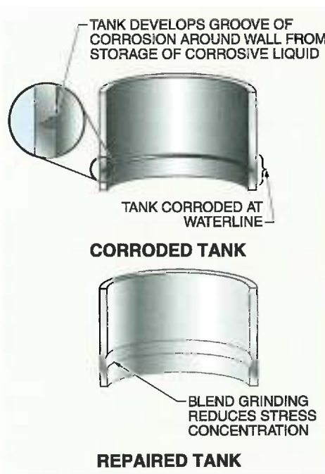
Figure 26-7. Blend grinding can be used to repair tanks in which corrosion has developed, and is an adequate repair if the remaining tank wall has sufficient structural strength. Blend grinding helps to prevent weld repair buildup on the surface.
