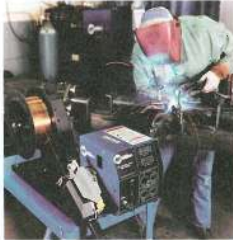
Figure 28-13. With a portable GMAW welding gun, the gas, current, and wire feed automatically begin to flow when the trigger is pressed.
