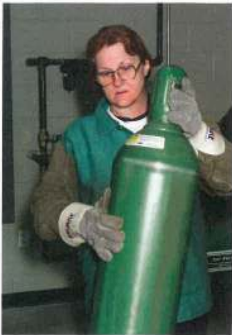
Figure 4-5. To safely move a cylinder, tilt the cylinder backward with one hand and roll the cylinder, guiding the cylinder with the other hand.
