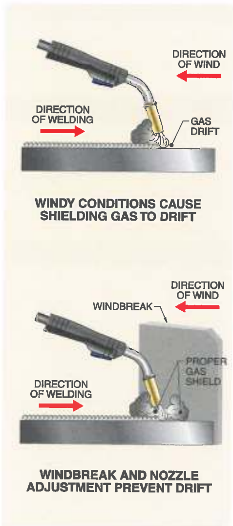
Figure 19-10. High travel speeds and windy conditions can cause the shielding gas to drift away from the arc. Windbreaks or moving the nozzle closer to the weld can help control drift.
