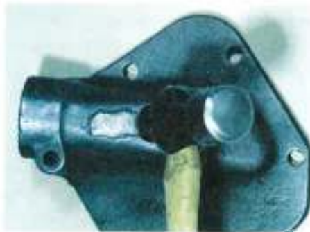
Figure 40-6. Careful joint preparation is required when welding cast iron.
