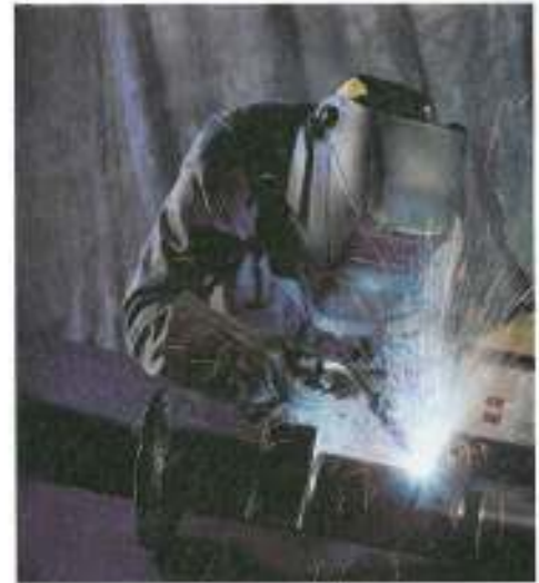
Figure 27-22. Gas metal arc welding is often used to join small-diameter pipe while the welder controls the welding gun.
