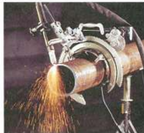
Figure 27-5. An oxyacetylene beveling machine can be used to bevel pipe.
