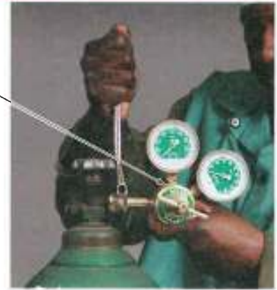
2 ATTACH OXYGEN REGULATOR AND HOSE
