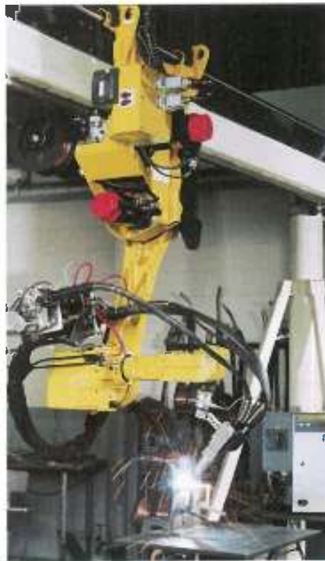
Figure 1-3. Robotic welding machines are programmed to perform repetitive welds on mass-produced products and require supervision by a skilled welding machine operator.
