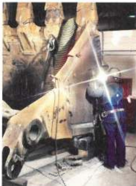
Figure 24-1. Surfacing is used on heavy equipment to retain the ductility of the base metal, while providing a surface resistant to abrasive wear.
