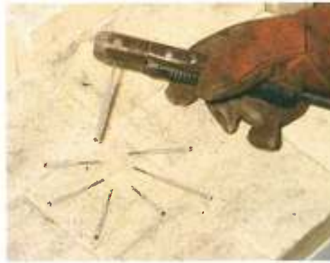
Figure 9-6. Use electrodes until the stubs have been consumed down to 1½" to 2" long.
