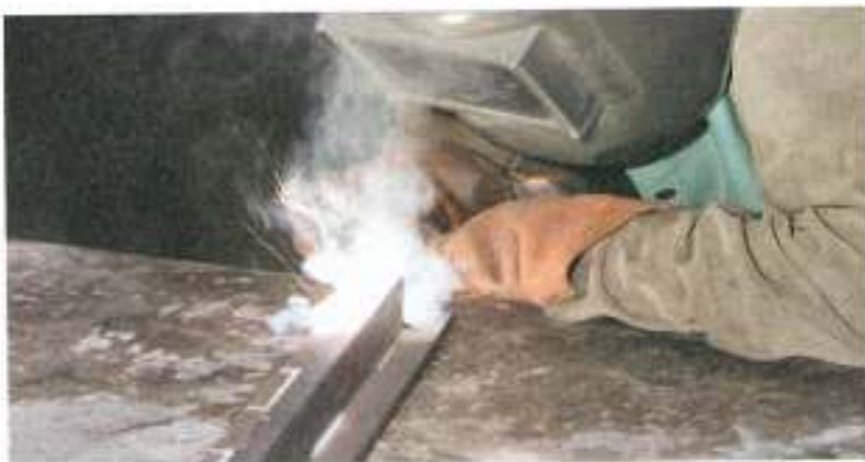
A welder performance qualification test qualifies a welder based on the essential variables specified on the welding performance qualification record.
