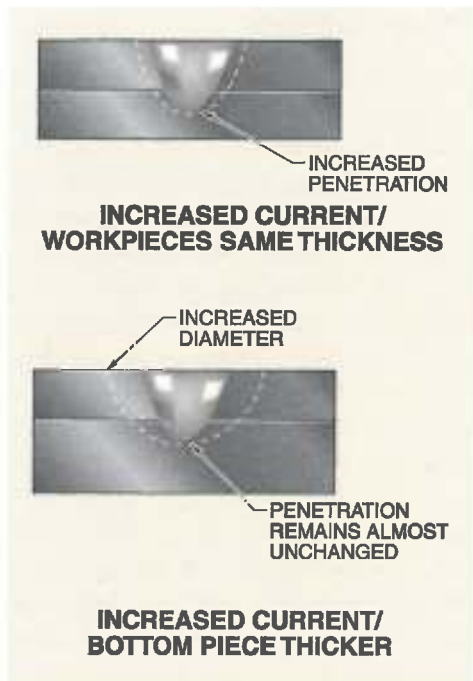
Figure 28-11. The thickness of the workpieces being welded has an effect on weld diameter and penetration when the current is increased.
