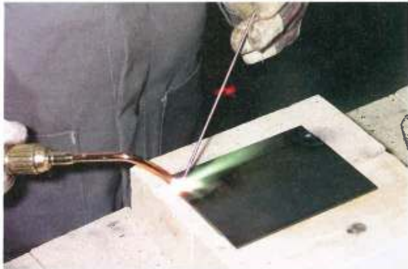
Using the correct size welding tip provides sufficient heat to melt the base metal for the required welding process.
