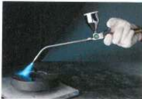
Figure 24-10. In flame spraying, a torch is used with the proper flame setting, and a trigger is pressed to propel the coating to the surface.
