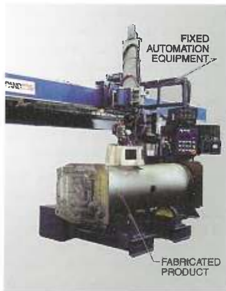
Figure 29-1. Fixed automation equipment is designed for a specific production function.
