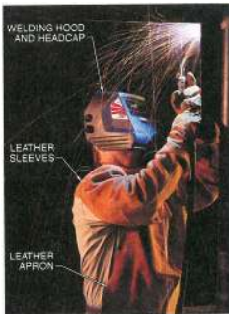
Figure 15-2. Proper personal protective equipment must be worn when performing overhead welding to prevent injury.
