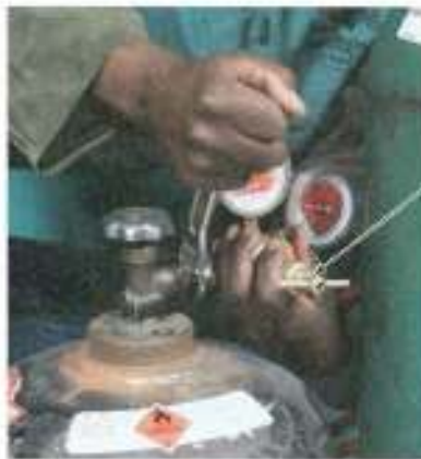
3 ATTACH ACETYLENE REGULATOR AND HOSE
