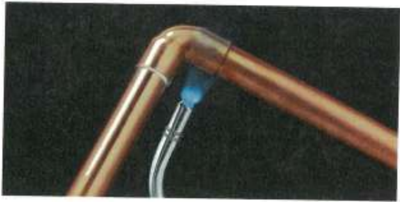
Copper tubing has high thermal conductivity and is commonly joined by sweat soldering. Thermadyne Industries, Inc.
