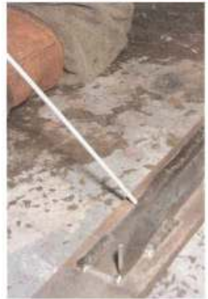
2 USE PROPER ELECTRODE ANGLE
