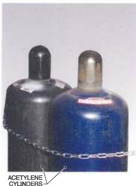
Figure 4-6. Cylinders should be chained at all times during use and when stored.
