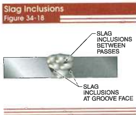
Figure 34-18. Slag inclusions are nonmetallic materials formed by slag reactions that are trapped in a weld. Slag inclusions can occur between passes or at the groove face.
