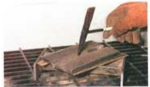
Figure 35-8. Interpass cleaning is required to remove slag from the weld and prevent slag inclusions.
