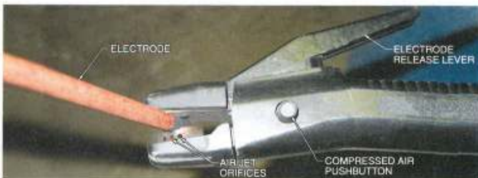
Figure 25-15. The carbon-graphite electrode must be held in a special electrode holder designed for air carbon arc cutting.
