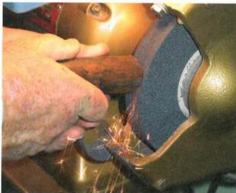
A grinding wheel is used for spark testing and should be kept clean to prevent contaminants from interfering with the spark stream.
