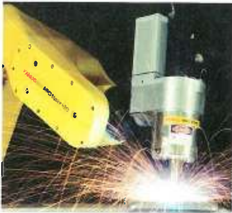
Figure 29-9. The GMAW process provides arc control and filler wire control to the robot simultaneously.
