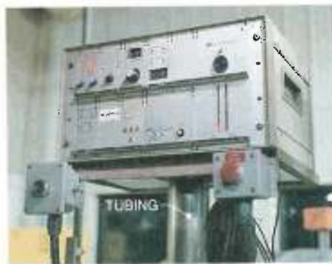
Figure 32-31. To inspect longitudinal weld quality in welded pipe or tubing, an energizing coil and a detector coil are required.
