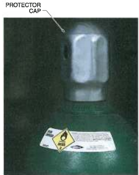
Figure 4-1. A protector cap screws onto the neck ring of the cylinder to protect the valve from damage when not in use.
