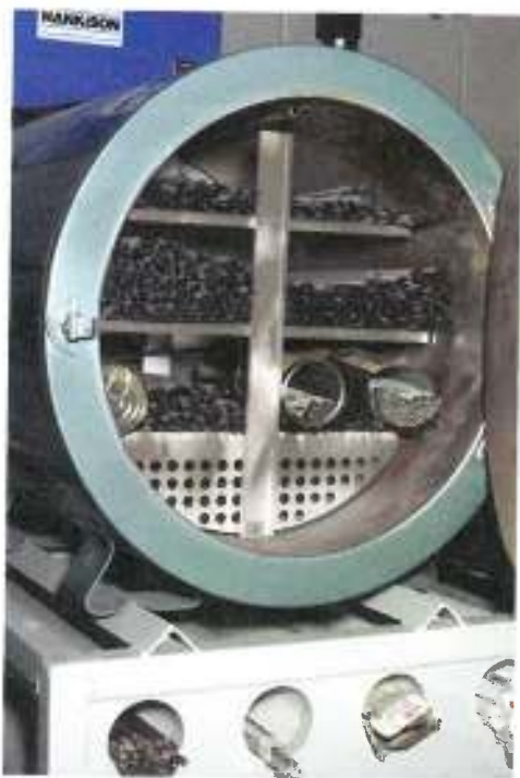
Figure 34-10. Low-hydrogen electrodes can help prevent underbead cracking. Moisture is removed from electrodes before use by storing the electrodes in an oven.
