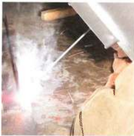
Figure 11-1. Heat from the arc melts the base metal, forming a crater into which molten base metal and filler metal can flow to create a quality bead.
