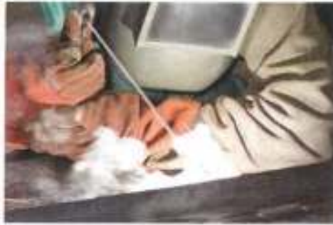
Figure 9-5. The electrode selected must be matched to the position of the weld joint.
