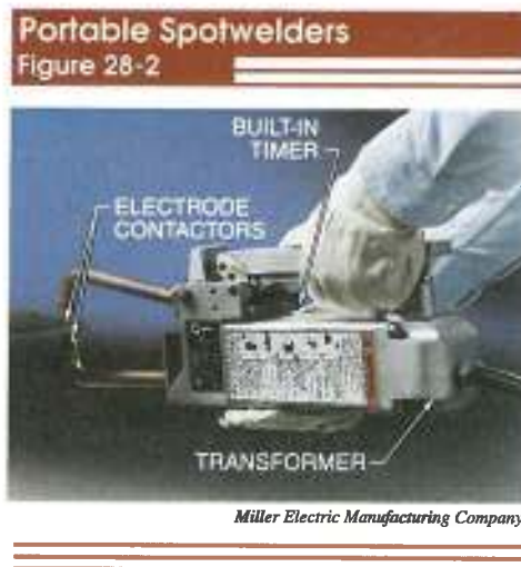
Figure 28-2. A self-contained portable spotwelder contains a built-in timer, electrode contactors, and a transformer.
