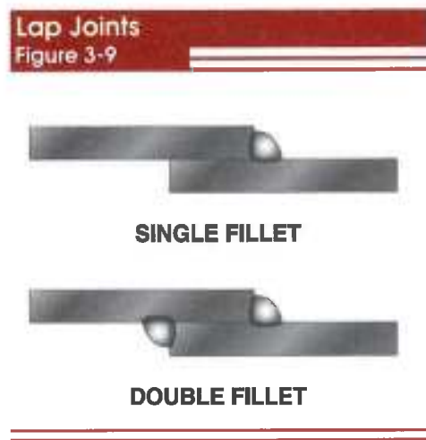
Figure 3-9. The single fillet and double fillet lap joints are the strongest weld joints available.
