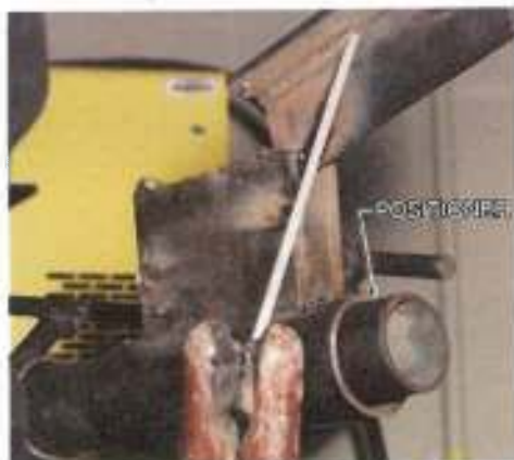
Figure 15-1. A positioner allows work to be adjusted to any height or position.
