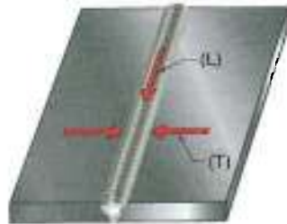
Weld Metal Shrinkage Figure 43-1
