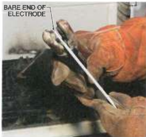
Figure 10-3. Place the bare end of the electrode in the electrode holder.
