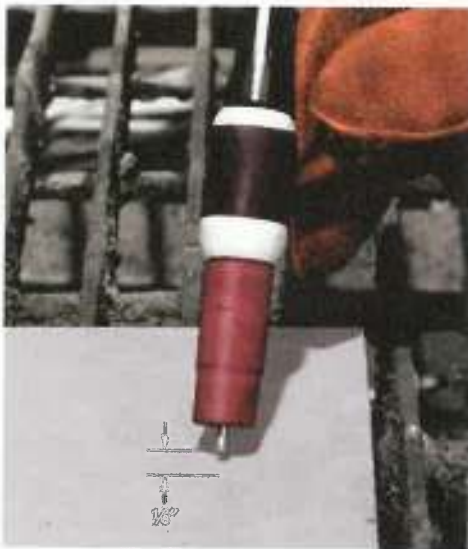
When starting the arc using AC, angle torch so electrode is 1/8" above workpiece. Current will jump gap and establish an arc.
