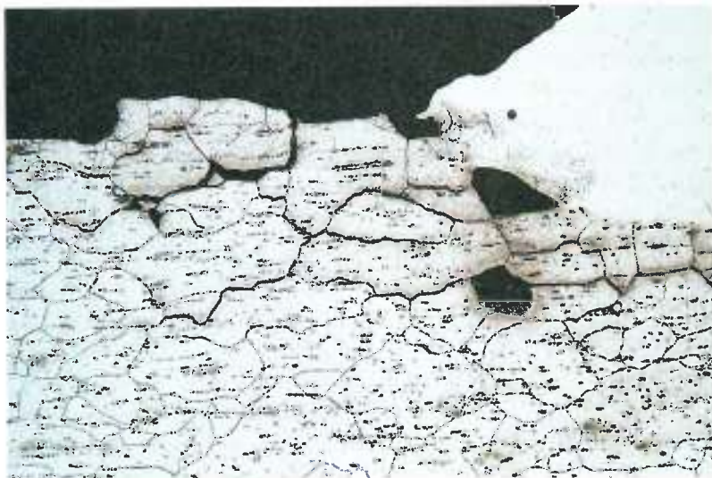
Magnetic particle examination may be used on a magnetic stainless steel to locate hot cracks near the surface of the weld.
