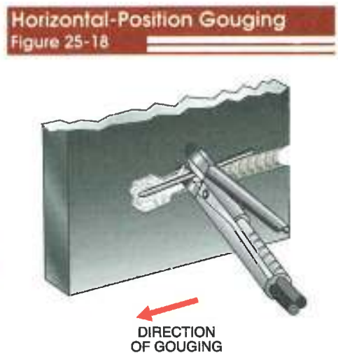
Figure 25-18. Gouging in horizontal position can be performed from either the left or the right. The air jet orifices should always follow the electrode.
