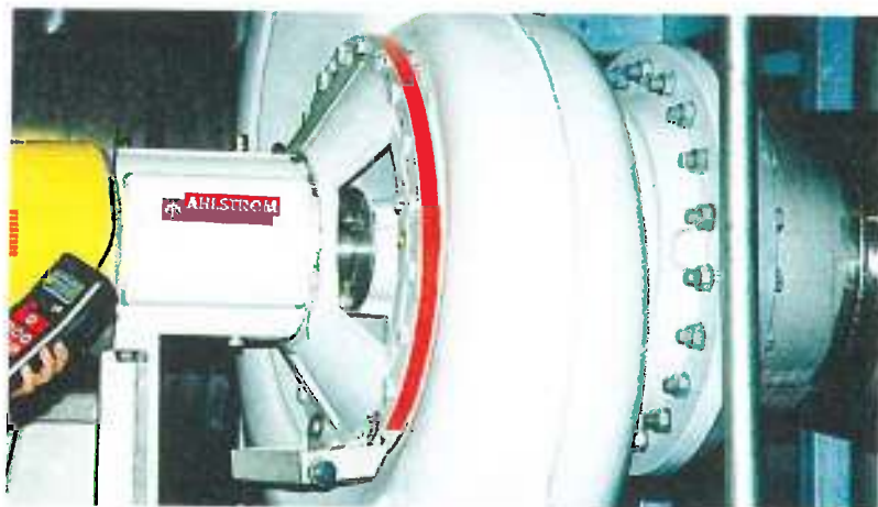
Ductile irons are commonly used for pumps in industrial applications.
