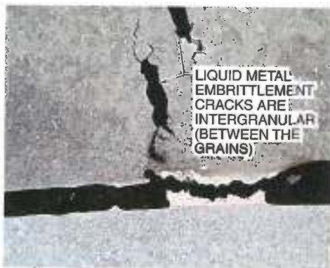
Figure 34-14. Liquid metal embrittlement commonly occurs in certain types of metals, usually where a part is exposed to excess stress.
