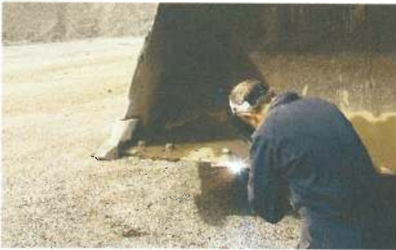
Construction equipment commonly uses surfacing welds with SMAW for building up worn parts and producing a hardened surface.
