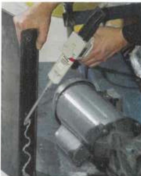
Figure 28-26. Adhesive bonding is used to join dissimilar materials and strengthen joints prone to failure from vibration.
