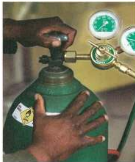
Figure 5-3. Stand to one side of the regulator when opening a cylinder valve.
