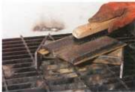
② REMOVE REMAINING SLAG WITH WIRE BRUSH
