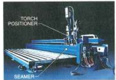
Figure 29-2. A torch positioner used on a seamer keeps the torch on a linear path along the joint and maintains a constant speed.
