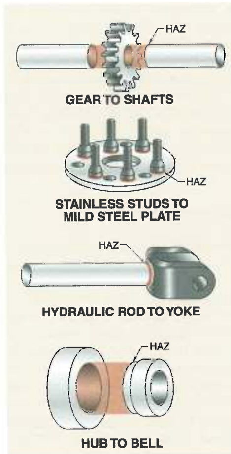
Figure 28-18. On friction-welded workpieces, the HAZ is confined to a very narrow band.
