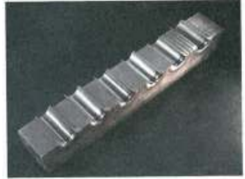
Figure 35-12. A mock-up is used for a mock-up test to simulate actual production welding situations to ensure proper tooling and techniques are selected, such as for heat exchanger tube-tubesheet joints.
