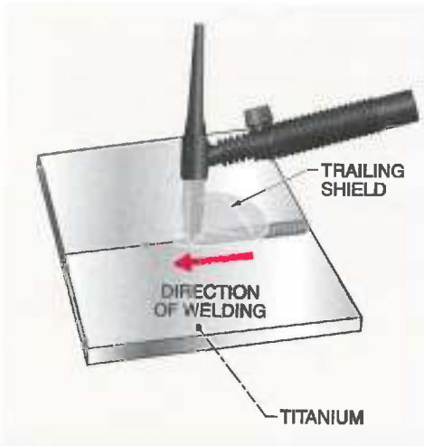
Figure 42-9. The metal cooling from welding temperature must also be protected by a trailing shield.
