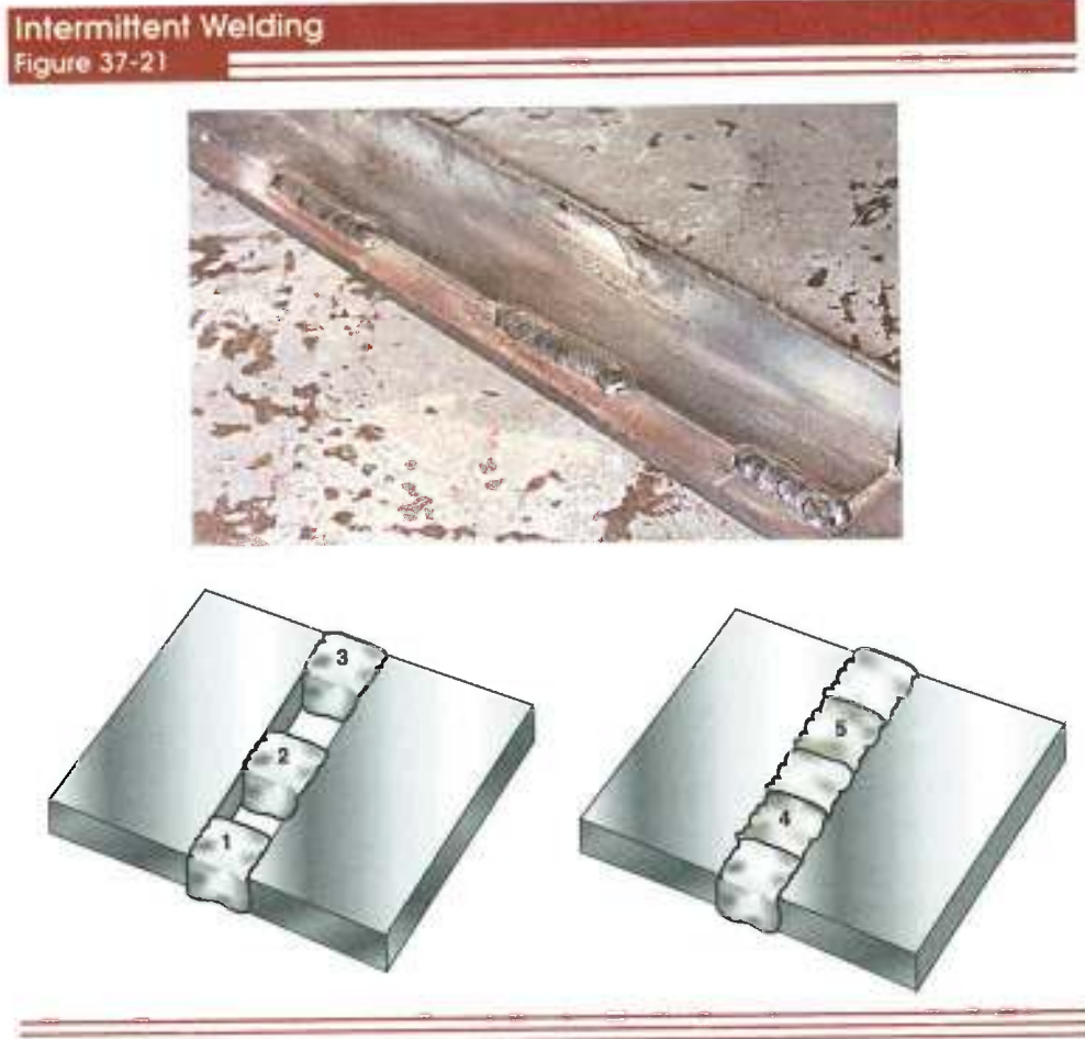
Figure 37-21. An intermittent weld can be used to prevent distortion by minimizing heat input.
