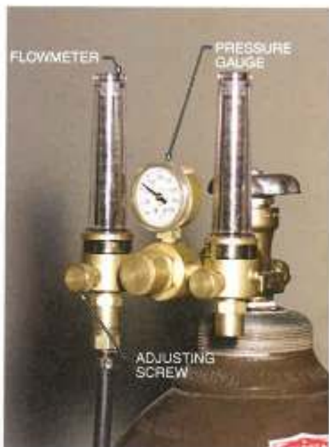
Figure 16-15. A pressure regulator and flowmeter control the flow of shielding gas to the torch.
