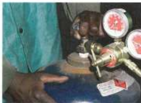
Figure 4-3. The acetylene cylinder valve should be opened with the installed valve handle.
