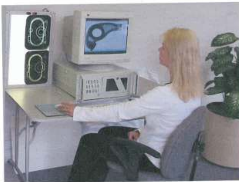
The results of radiographic testing are downloaded to a computer for storage and future reference.
