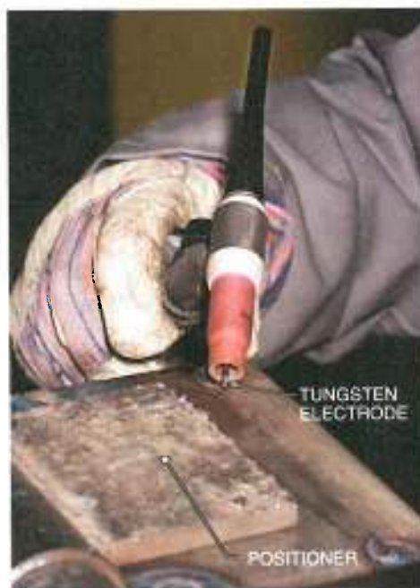
Figure 16-12. In GTAW, a tungsten electrode is used to provide the arc for welding; it is not consumed in the weld.
