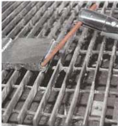
Figure 25-20. When beveling a plate, hold the electrode at a 45° angle.
