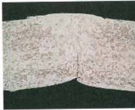
Figure 20-14. Lack of penetration can result from low heat input to the weld area or a failure to keep the arc located properly on the leading edge of the weld pool.
