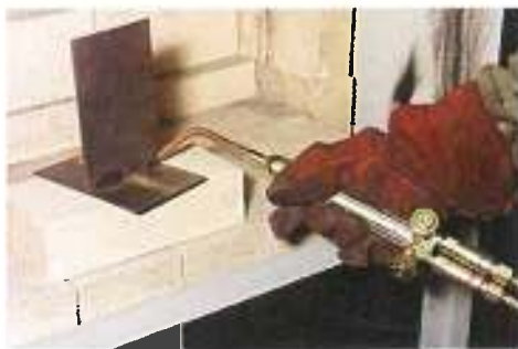
Figure 6-1. When welding light-gauge metal in flat position, grasp the torch like a hammer.
