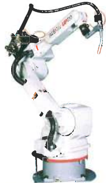
Figure 29-4. A common configuration for a welding robot is a six-axis articulated robot manipulator.
