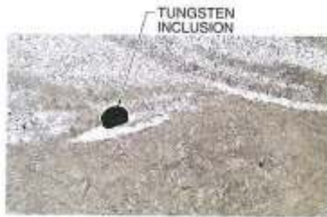
Figure 34-21. Tungsten inclusions are particles found in the weld metal as a result of the nonconsumable tungsten electrode coming in contact with the work or the molten metal.
