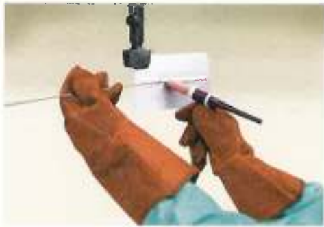
Figure 17-7. Dip the filler metal into the high side at the front of the weld pool when welding a horizontal butt joint.
