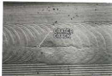
Figure 20-13. Crater cracks can occur if the welding gun is removed before the weld pool has solidified.
